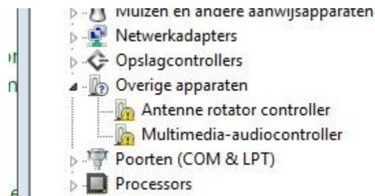
Right click on the line that shows “Antenne rotator controller” and select update driver.
