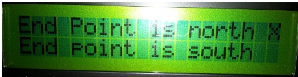
Use the CCW and CW buttons to move the X. Use the SET button to save this setting.
