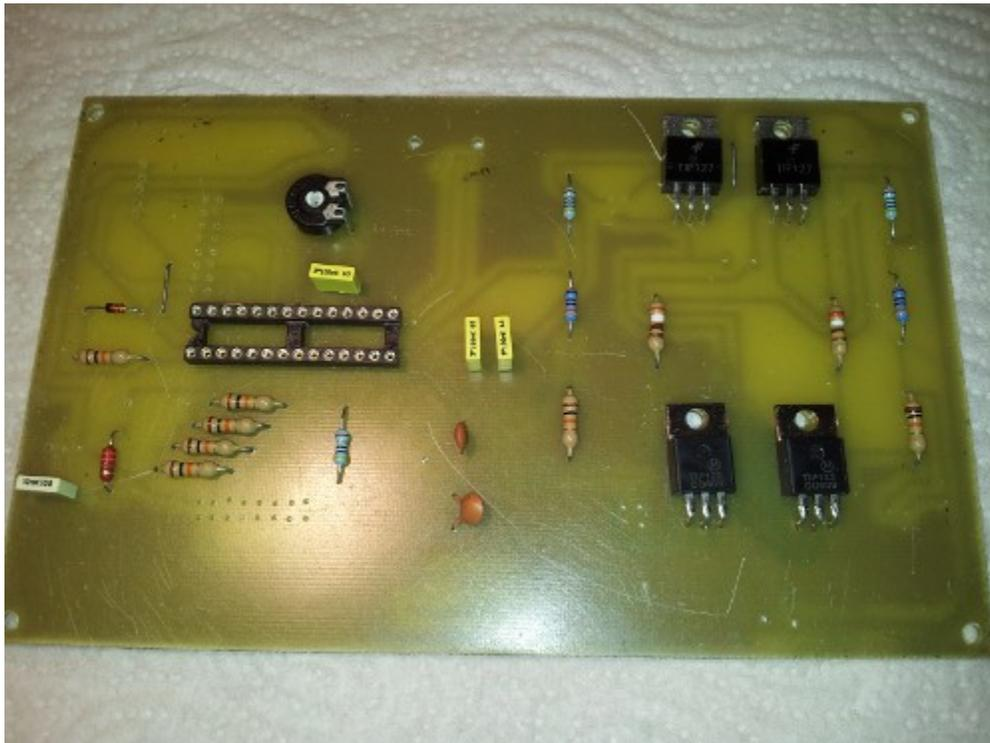
As my motor only needs a current of 0.7 amps, cooling of the Darlington transistors was not needed.
