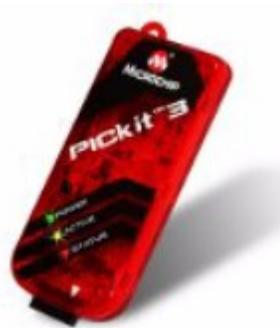
The PICKit3 has a 6 pins connector that will fit the 5 pins program header on the main board. The white down arrow should be connected to the 1<sup>st</sup> pin of the program header, leaving the last pin free on the PICKit3.
