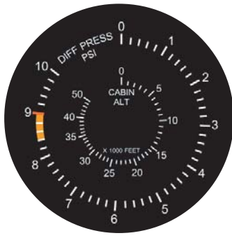
Cabin Climb indicator dual needle
