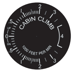
Cabin Climb indicator single needle
