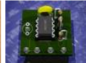
Render 3D images of your PCBs using Eagle3D and POV-Ray by ongissim
